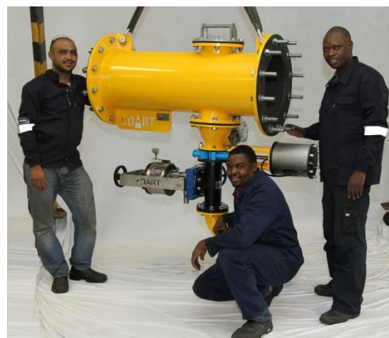
The cutter design promotes flow recovery downstream of the cutter.
